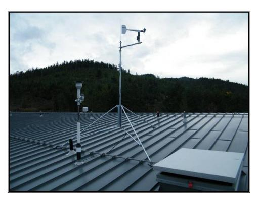
Figure 4 Tripod Mounted Anemometer and BAM Inlet located on the Roof of the HPC building
