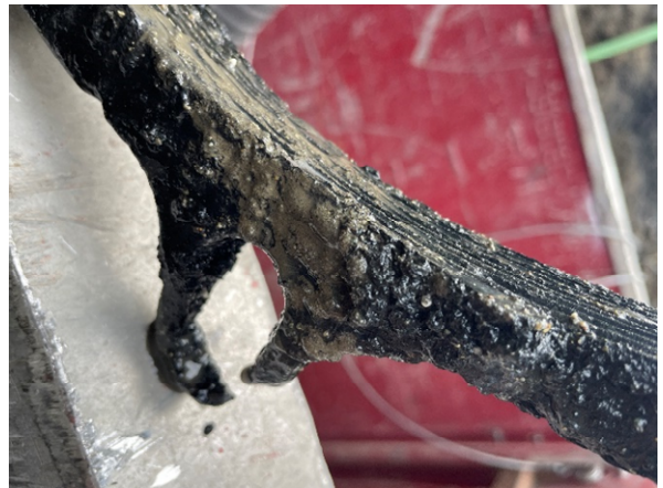
Photo 4 - Corroded Restraining Ring Ear.
