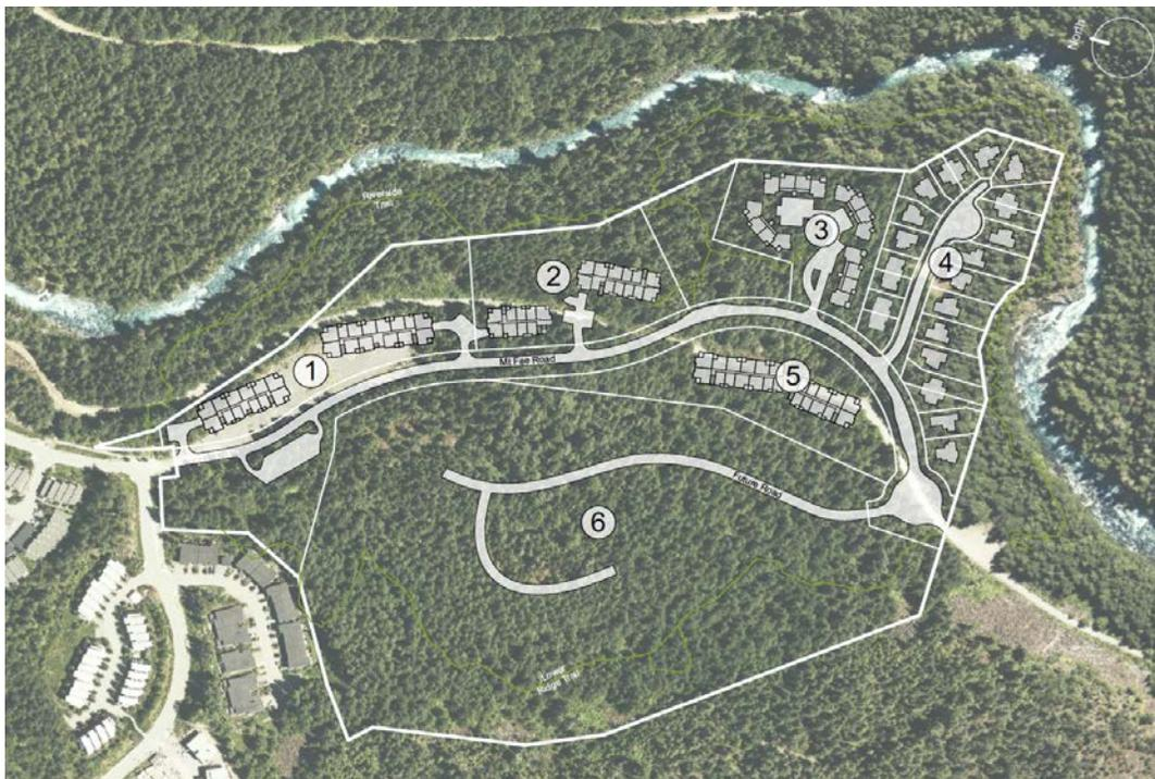
Both building sites on Lot 2 have all underground services stubbed to the property line, ready for construction. In 2022 WDC also completed all bulk blasting and excavation for both buildings. Detailed excavation, structural fill (2B) and foundation preparation will continue through the winter to ensure at least Building 2A is ready for construction by March 2023. The site has generally been prepared for site offices, sub-trade site offices, construction power and crane pad preparation.
