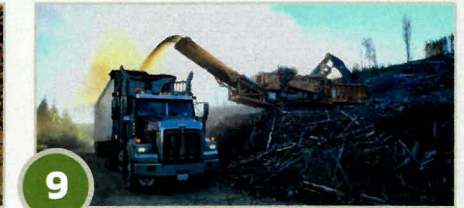
9 Slash Grinding. Led by Valley Carriers Ltd., 24,000 cubic metres of wood waste was ground in the forest with special equipment and transported to Merritt Green Energy to be converted to electricity. Photo Credit: Valley Carriers Ltd.
