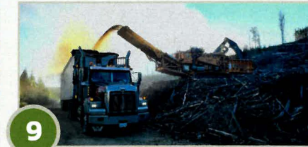
9 Slash Grinding. Led by Valley Carriers Ltd., 24,000 cubic metres of wood waste was ground in the forest with special equipment and transported to Merritt Green Energy to be converted to electricity. Photo Credit: Valley Carriers Ltd.
