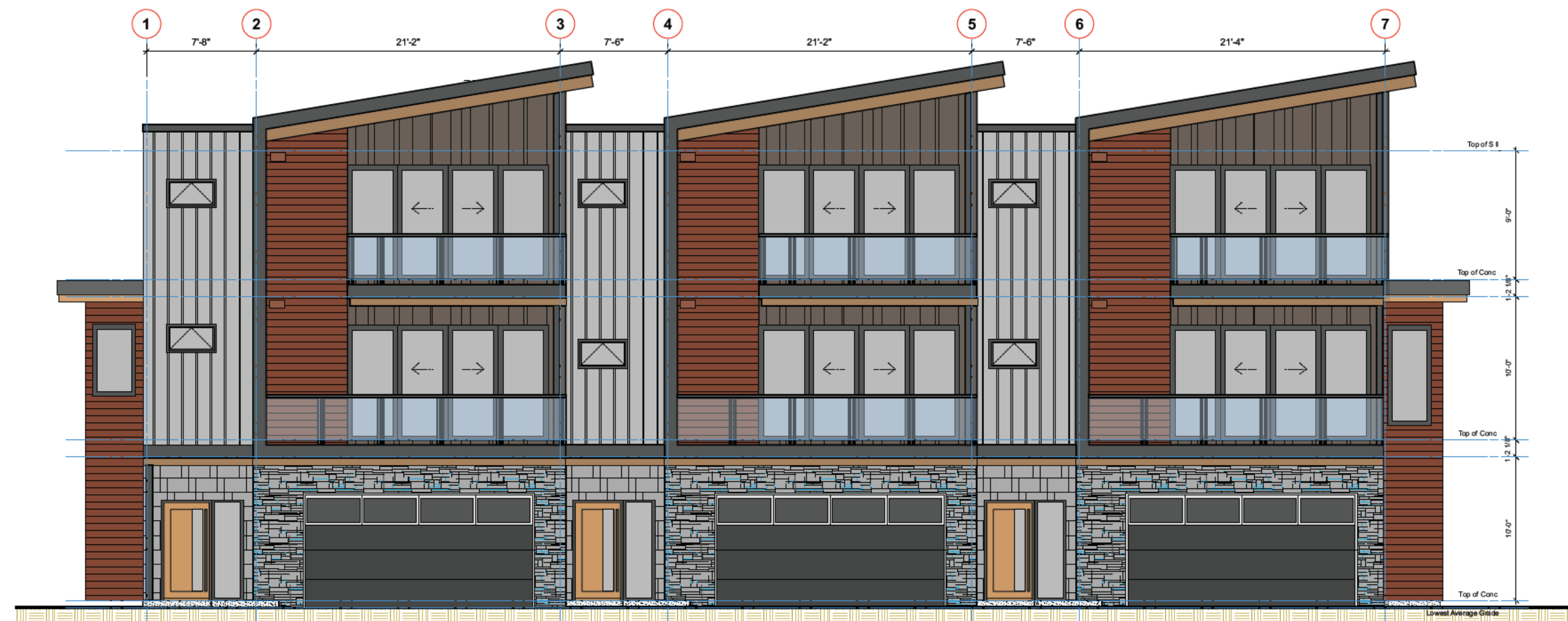
1 BUILDING C/D - TRIPLEX - FRONT ELEVATION A-3.1 1/4" : 1'-0"
