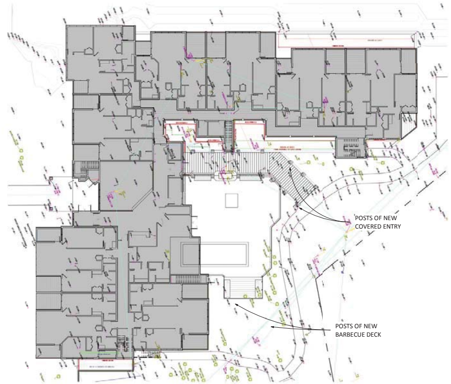
2 DP 1.3 1" = 30'-0" 1ST FLOOR PLAN - SITE COVERAGE - PROPOSED - 29.06%
