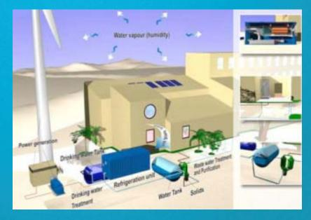
The AWG technology allows water to be produced at any location in the world. It is independent of stationary water resources. The economic benefit is enhanced by the fact that cold air generated in the condensation process can be used for air-conditioning buildings.
