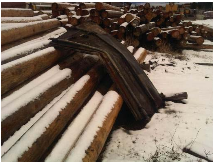
The photo above shows the bending of one of the container doors that was blown off in the explosion.
