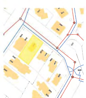
SHOWING SANITARY AND WATER SERVICE ALONG KAREN CRESCENT
