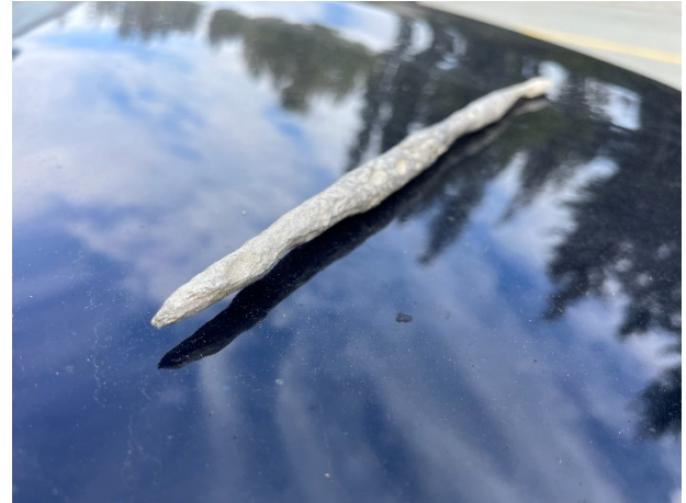
Photo 2 - Corroded Restraining Rod (S2-16 22.5° Bend)
