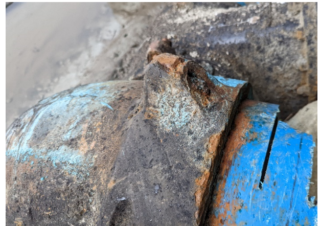
Photo 2 - Corroded 90° Bend Restraining Ear.
