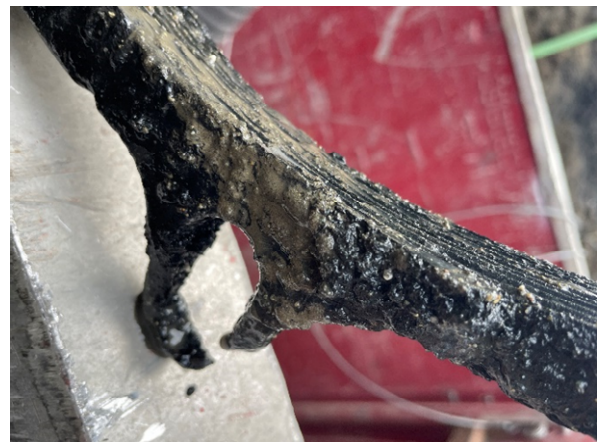
Photo 4 - Corroded Restraining Ring Ear.
