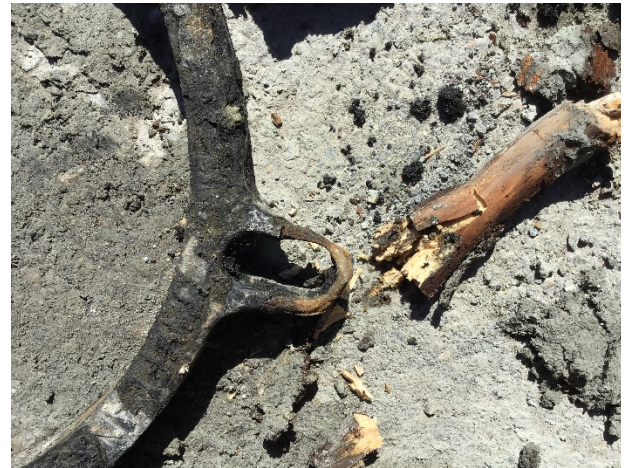
Photo 2 - Corroded Restraining Ring Ear.
