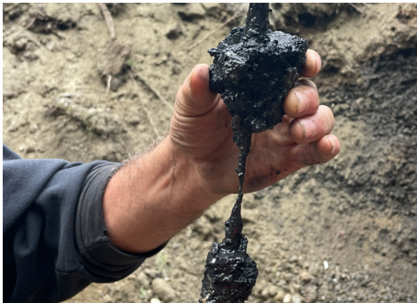
Photo 1 - Corroded Restraining Rod.
