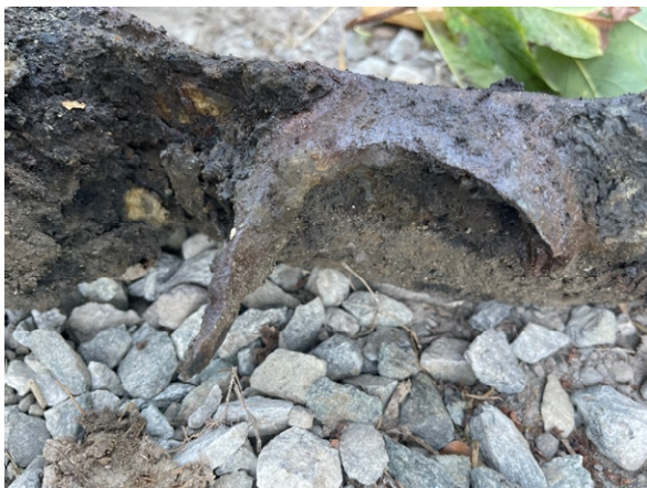
Photo 3 - Corroded Restraining Ring Ear.
